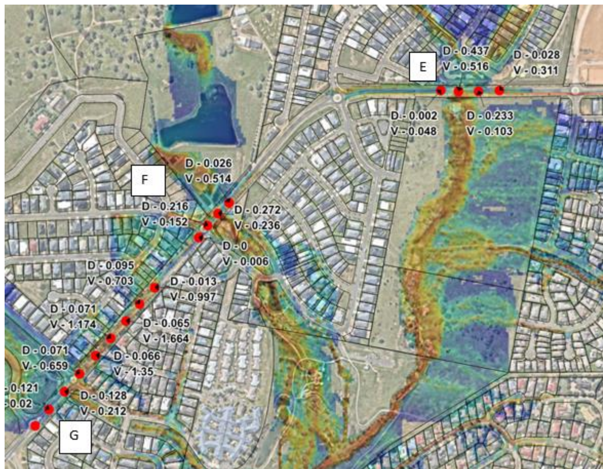
Figure 15 – Evacuation Route 1% AEP via Marys Mount Road Points E - G
